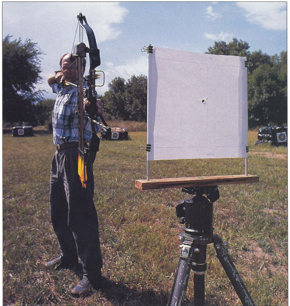
This paper holding device allows the shooter to tune the bow easily in the field. Set the paper far enough from the shooter so that the arrow will just clear the bow before striking the paper. Proper shooting technique is extremely important.
